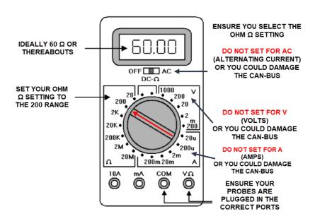
The above diagram is shown as a guide but your meter may be different, in which case please refer to your meter user guide for how to test within the 200 ohm range.
