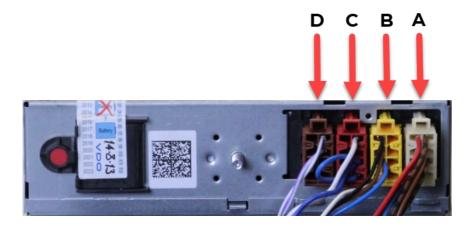
These diagram shows the four ports at the back of the tachograph which are from right to left A, B, C and D.
