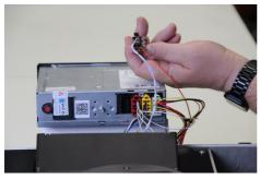
If there is already a wire fitted to the D plug pin 8 then the DOT Orange needs to be joined to that wire. This can be done by splicing and soldering or replacing the in.
