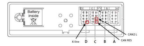
Also important are the pins 7 and 8 on the C port and pin 8 on the D port.
