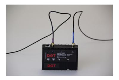
Please ensure that the GPS antenna has a clear sky view and has the black plastic side facing the sky. The GSM antenna must not be attached to metal to ensure a better signal.
