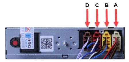
You require access to the back of the tachograph to where the A-D sockets are situated.
