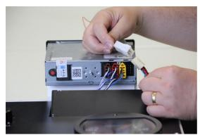
Connect the same A connector to the DOT loom white socket
