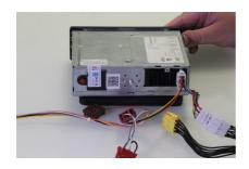
Then plug the DOT loom 'A' Connector into the tacho.
