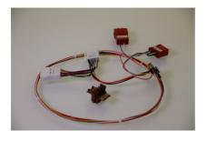
2) The DOT wiring loom which includes a separate brown plug which may be required
